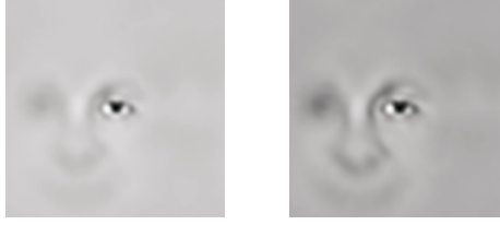
Fig. 4. Comparison of the visual appearance of an ASEF filter (left) and the combined PSEF filter (right). Both images show “right eye” filters with shifted quadrants.
