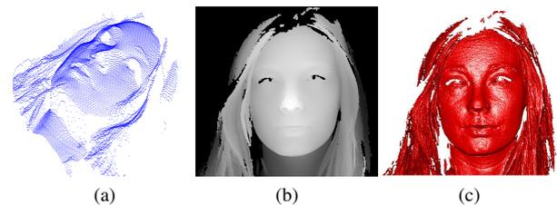
Figure 4. 3D data representation: (a) point cloud, (b) depth image, (c) shaded depth image.
