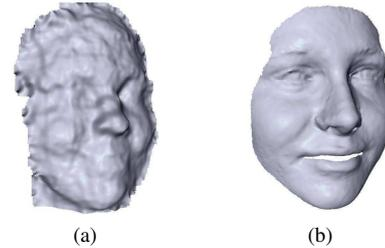
Figure 3. 3D face image acquired by the Kinect sensor: (a) raw image, (b) adapted 3D face model.
