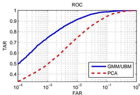
Figure 8. ROC curve of the proposed system compared to the global PCA approach.
