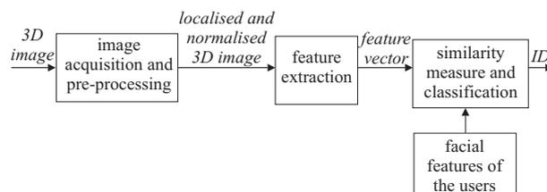
Figure 1. Block diagram of a 3D face-recognition system.
