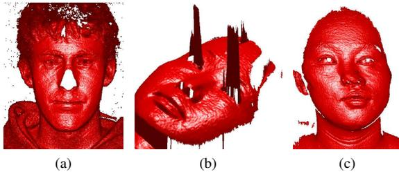
Figure 2. Examples of scans with distortions: (a) nose absence, (b) noise around the eye region, (c) distortion due to face motion during image acquisition.
