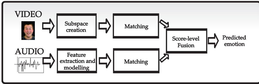
Figure 1. Block diagram of the multi-modal emotion recognition system
